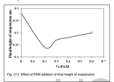
It is worth mentioning that the solid concentration of the untreated sludge = 152.8 kg.m<sup>-3</sup>. Taking into consideration that the specific gravity of the solids is about 2500 kg.m<sup>-3</sup>, this corresponds to a volumetric concentration of approximately 0.061 m<sup>3</sup> solids per m<sup>3</sup> water. Since the total volume of solid is constant, the following equality can be set between the initial conditions (0) of the suspension and its final conditions (f):
