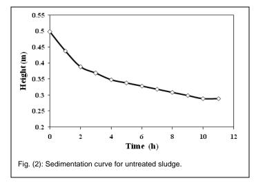
The initial rate of settling as calculated from the numerical value initial of the slope of the curve was found to equal 0.0547 m.h<sup>-1</sup>. The final asymptotic height of interface was about 0.288 m.
