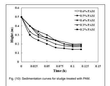
As for the final height of suspension, the addition of PAM drastically reduces that height, therefore increasing the amount of settled solids. As can be followed in Figure (11), adding PAM has for effect to reduce the limiting height of suspension from about 0.29 m in case of untreated sludge to less than half that value upon adding 0.2% PAM. Increasing the polymer addition is accompanied by a slight increase in that height.
